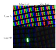
Array repair – block removal
