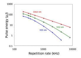
High-power PicoBlade typical pulse energy versus repetition rate for 1064, 532, and 355 nm\*
