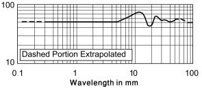
Fig. 6. Spectral response of  $\mathsf{Pyrocam}^{\mathsf{TM}}$  III detector array without window.
