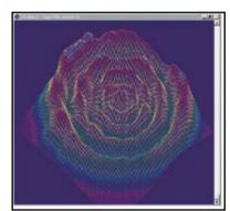
Nd:YAG laser with cavity misalignment. Pyrocam, such as the analysis of excimer
