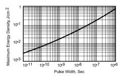
Pulsed damage threshold of pyroelectric detector coating.
