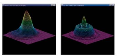
CO<sub>2</sub> laser with cavity misalignment.
