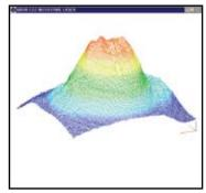
Fig. 2. Beam profile of industrial CO<sub>2</sub> laser making consistently good product.
