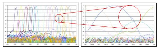
dBm Optics uses a patented technique to rapidly determine the correct measurement range, change to that gain, forcibly inject or deplete charge from the amplifiers (to force rapid settling), then make the measurement. All this (including the measurement) takes less than 10 µs. Our intra-range linearity is assured using a special calibration technique that occurs in the background.
