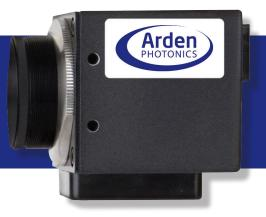
The BQM-10 laser beam profiler range is a high precision, CCD and InGaAs based beam profilers for use with lasers with wavelengths between 400 and 1700 nm. Allied with our powerful but intuitive software packages, the BQM-10 range makes quick and accurate characterisation of your lasers a reality.
