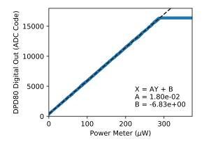
Figure 7: Digital ADC power calibration. Low gain mode.
