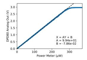
Figure 9: Analog output power calibration. Low gain mode.  $^{3}$
