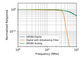
Figure 5: Frequency response of the DPD80.<sup>2</sup>
