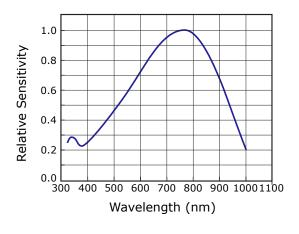
Figure 10: Spectral sensitivity
