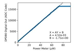
Figure 6: Digital ADC power calibration. High gain mode.
