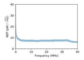
Figure 3: Digital noise floor at 1 kHz BW. Low gain mode.
