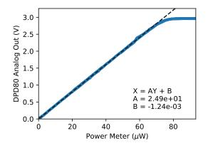
Figure 8: Analog output power calibration. High gain mode.  $^{\rm 3}$
