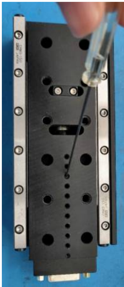
Old style limits, adjust with a 0.05in allen(or hex) wrench
