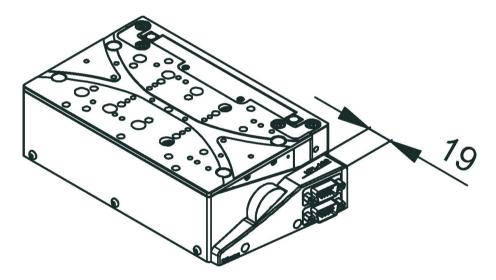
UPL-120, stepper motor, dimensions in mm
