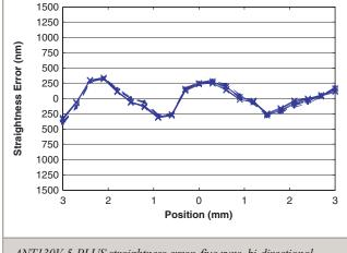
ANT130V-5-PLUS straightness error, five runs, bi-directional, perpendicular to the wedge.
