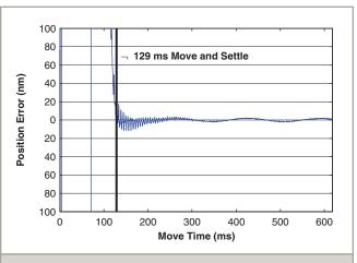
ANT130V-5-PLUS step and settle performance at 75 mm/s, with a settle spec of ±20 nm, and a step size of 5 mm. Outstanding settling time enhances throughput of most applications.
