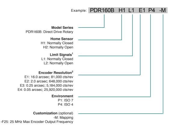
Notes: 1) The PDR series does not include limit sensors. The Limit Signal options are provided for compatibility with motion controller requirements. 2) Standard encoder max output frequency is 12.5 MHz. Not all configurations are valid - consult factory for assistance
